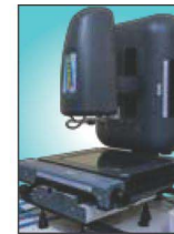
Vision Measurement System (Precise incoming component inspections)
